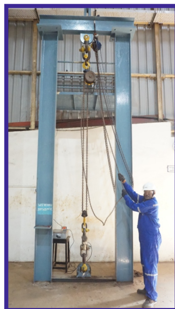
Vertical Test Bench SWL : 30 MT, Height : 5.2 mtr
